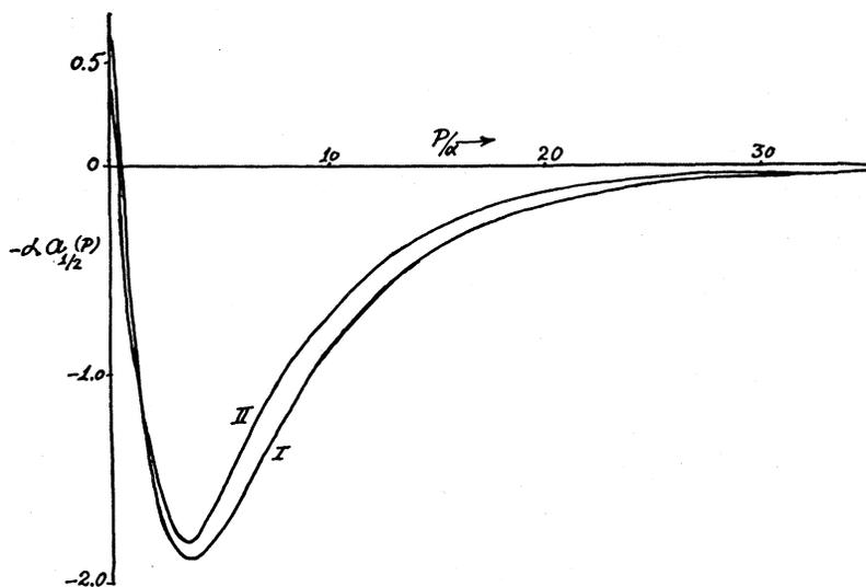
FIG. 4. Amplitude  $-\alpha a_{1/2}(P)$  as a function of  $P/\alpha$  for  $k_i=0$ . Curve I corresponds to the case  $\beta_1=\beta_2=6.255\alpha$  (Yamaguchi, Ref. 5) and curve II refers to the parameters  $\beta_1=5.8\alpha$ ,  $\beta_2=5.5\alpha$  (Naqvi, Ref. 6).
