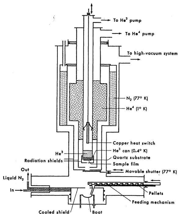
FIG. 1. Dewar for tunneling measurements on alloy films evaporated at low temperatures.
