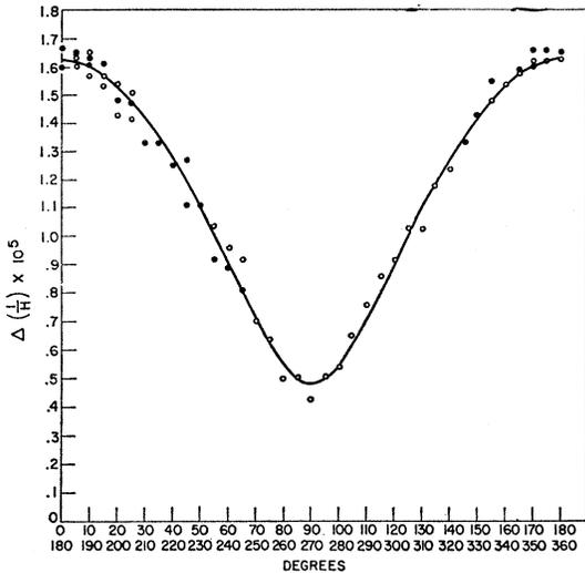
FIG. 5. Observed hole periods as a function of magnetic field angle for *H* in the *y-z* plane and *I* || *x*. The curve is the result of a least-squares fit.
