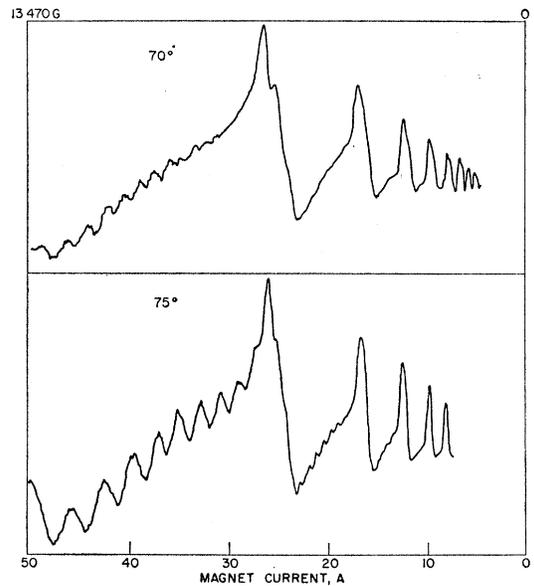
FIG. 7. Experimental curves for *I* || *y* *H* at 70° and 75° from the *z* axis. Note how the second harmonic appears abruptly for a change of only 5° in magnetic field angle. In addition, note the spiky character of the electron peaks.
