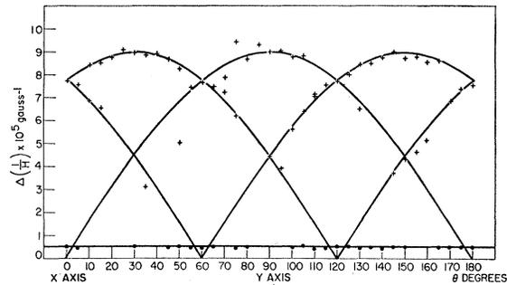
FIG. 4. Observed periods as a function of magnetic field angle for  $H$  in the  $x$ - $y$  plane and  $I||z$ . Crosses are low-field data (700–2000 G), while circles are high-field data. The two upper curves are for electrons and the lower one is a hole curve. The curves are those derived from least-squares fits.
