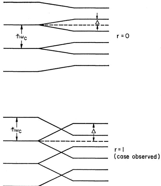
Fig. 1. Energy level of an electron in a magnetic field including spin for the case of  $\Delta = (\hbar\omega_c/4)$  (upper diagram) which corresponds to  $H$  being  $5^\circ$  from the  $y$  axis in the  $y$ - $z$  plane. The lower diagram is the case  $\Delta = \frac{3}{2}\hbar\omega_c$  corresponding to  $H$  being  $20^\circ$  from the  $y$  axis in the  $y$ - $z$  plane. In both cases one expects to see only the second harmonic.
