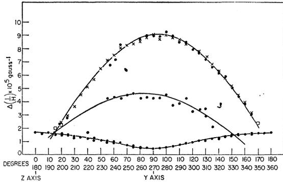
FIG. 2. Observed periods as a function of magnetic field angle for  $H$  in the  $y$ - $z$  plane and  $I||x$ . Crosses are low-field data (700–2000 G), while circles are high-field data. Squares represent periods derived from analysis of beat periods. The two upper curves are for electrons and the lower one is a hole curve. The curves are those derived from least-squares fits.
