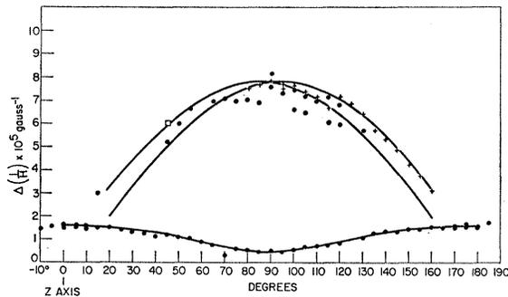
FIG. 3. Observed periods as a function of magnetic field angle for  $H$  in the  $x$ - $z$  plane and  $I||y$ . Crosses are low-field data (700–2000 G), while circles are high-field data. Squares represent periods derived from analysis of beat periods. The two upper curves are for electrons and the lower one is a hole curve. The curves are those derived from least-squares fits.
