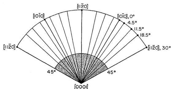
FIG. 1. The stereogram presented in Ref. 2 showing the magnetic field directions for which open orbits appear to exist in thallium.
