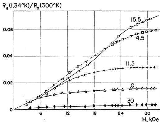
FIG. 2. Resistivity versus field strength for a thallium sample having its axis parallel to  $[0001]$  and the field in various directions in the basal plane. The angles are those between the magnetic field direction and the  $[10\bar{1}0]$  axis. (Taken from Ref. 2.)
