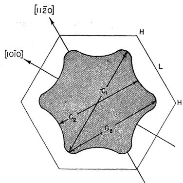
FIG. 6. The third zone sheet in the *AHL* plane. The dimension lines refer to the extremal calipers of the surface.
