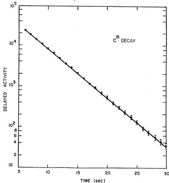
FIG. 4. Activity of  $C^{15}$ , produced by  $C^{14}(d,p)C^{15}$  reaction at 2.0 MeV. The solid curve represents a half-life of 2.49 sec; a half-life which differs from this by  $\pm 0.1$  sec leads to curves which lie well outside the error bars associated with the experimentally observed points beyond  $t=15$  sec.
