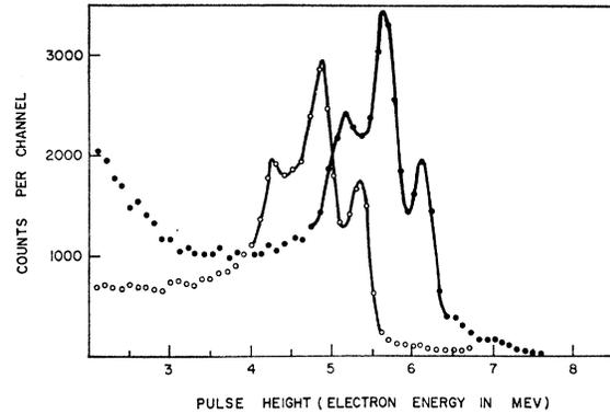
FIG. 3. Spectra of delayed activity produced in a 3- $\times$ 3-in. NaI crystal by C<sup>15</sup> (open circles) and N<sup>16</sup> (dots). Observed similarity of curves is expected on basis of decay schemes (see Fig. 1); this similarity complicates separation of activities.
