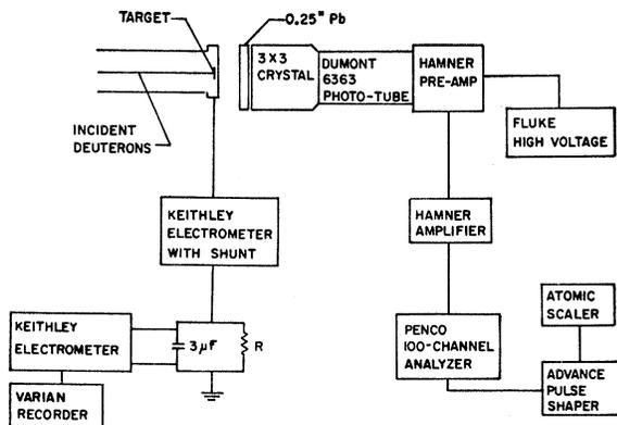
FIG. 2. Block diagram showing arrangement of detecting and counting apparatus. Delayed activity of the target was recorded by using the multichannel analyzer in its time mode. Instantaneous charge on the target was also measured and recorded.
