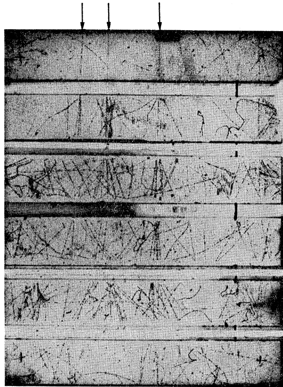
FIG. 1. Three typical 1000-MeV showers as observed in the five-plate cloud chamber.
