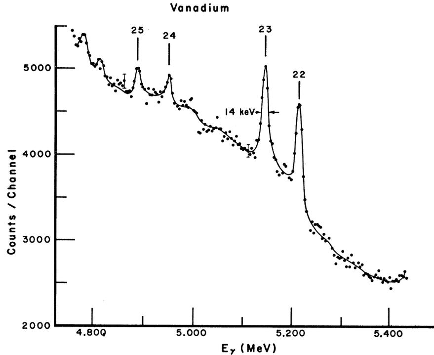
FIG. 6. Vanadium  $\gamma$ -ray spectrum observed with a gain of  $\sim 3.5$  keV/channel for  $4.85 \leq E_\gamma \leq 5.45$  MeV.
