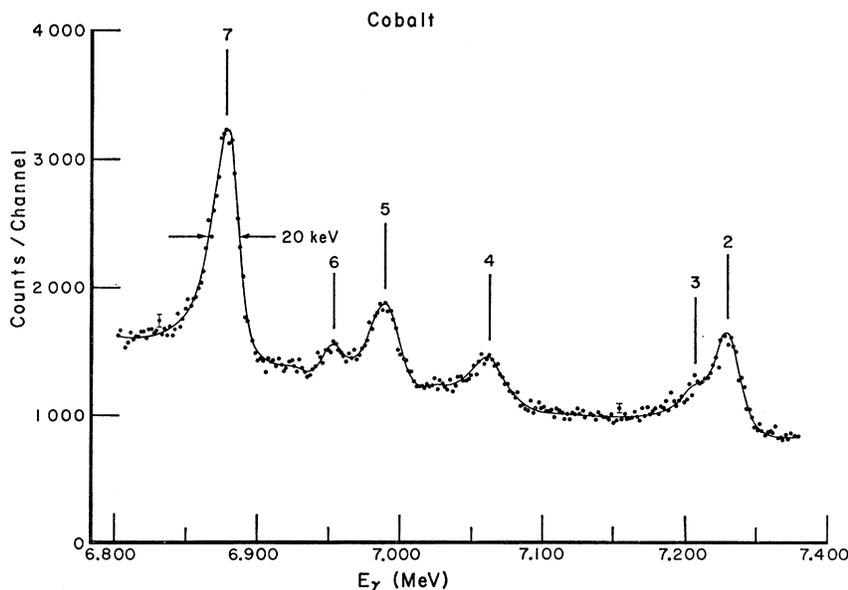
FIG. 14. Cobalt  $\gamma$ -ray spectrum observed with a gain of  $\sim 1.7$  keV/channel for  $6.80 \leq E_\gamma \leq 7.30$ . The bump on the low energy side of peak 2 is the evidence for the existence of transition 3.
