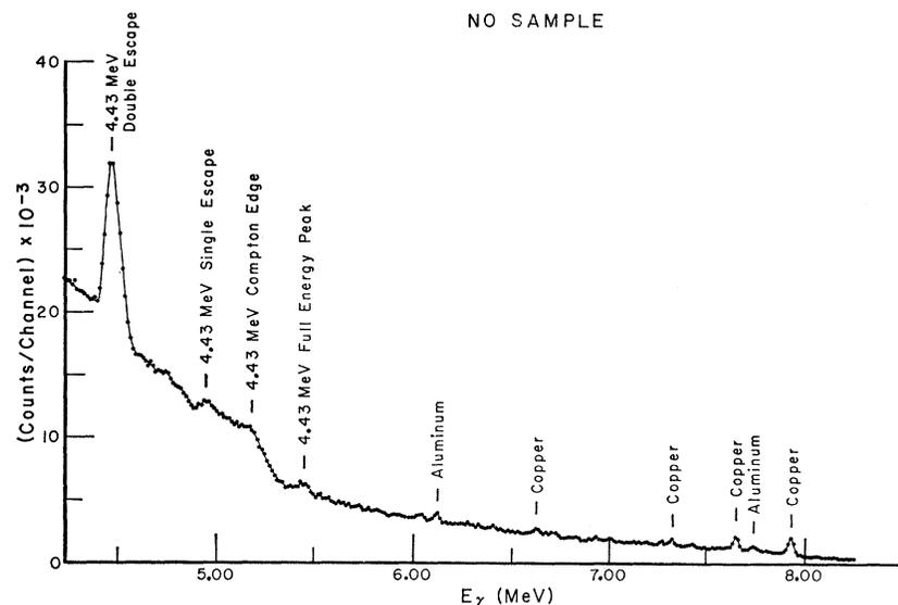
FIG. 2. The  $\gamma$ -ray spectrum observed with a gain of  $\sim 14$  keV/channel with no sample in place. Note the energy scale associates the full  $\gamma$ -ray energy with the 2-photon escape peak.
