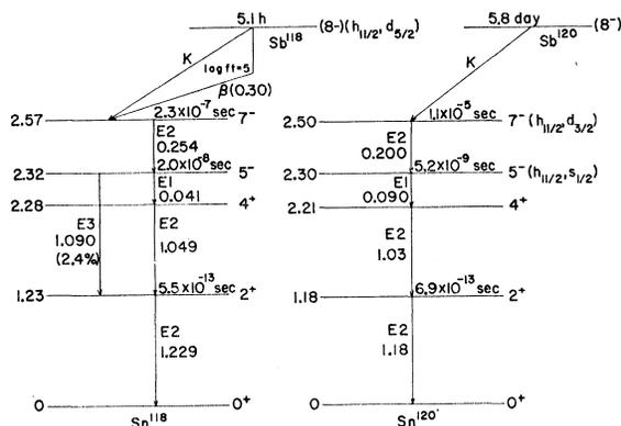
FIG. 14. Proposed decay scheme of  $\text{Sn}^{118}$  and  $\text{Sn}^{120}$  populated from the decay of 5.1-h  $\text{Sb}^{118}$  and 5.8-day  $\text{Sb}^{120}$  (Ref. 6). All energies are in MeV.
