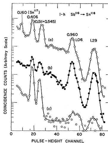
Fig. 2. Spectra in coincidence with (a) the  $K$  x ray, (b) the 0.099-MeV  $\gamma$  ray and (c) the 0.140-MeV  $\gamma$  ray, recorded simultaneously. Chance coincidence contributions have been subtracted from each spectrum. No corrections for coincidences due to underlying Compton distributions have been made.
