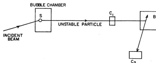
FIG. 2. Idealized experiment for measuring unstable particle decay. The interaction takes place in the sphere  $S$ ,  $C_1$  is a counter;  $B$  is a block of stopping material where decay occurs; and  $C_2$  is a recording counter.
