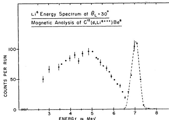
FIG. 3. Total energy spectrum of  $Li^{6+++}$  particles from the reaction  $C^{12}(d, Li^6)Be^8$ , obtained from 31 spectra of the type shown in Fig. 2. The width of the "sharp" peak reflects the target thickness rather than resolution of the detection system. The continuum is mostly due to  $Li^6$  ions from the 3-body breakup of the ( $C^{12}+d$ ) system. Errors shown are statistical. The dashed line marks the ground-state peak.
