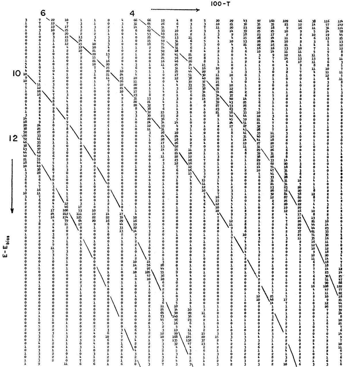
Fig. 6. Portion of the two-dimensional 128×32 channel analyzer printout, from a C<sup>12</sup>+d run at high counting rates (about 10<sup>4</sup> cps). The ordinate is proportional to (const-E) and the abscissa to τ≈(100 nsec-time of flight). Loci for masses 4, 6, 10, and 12 are sketched in to aid the eye. Run was taken with a 1-m flight path at θ<sub>L</sub>=12°.
