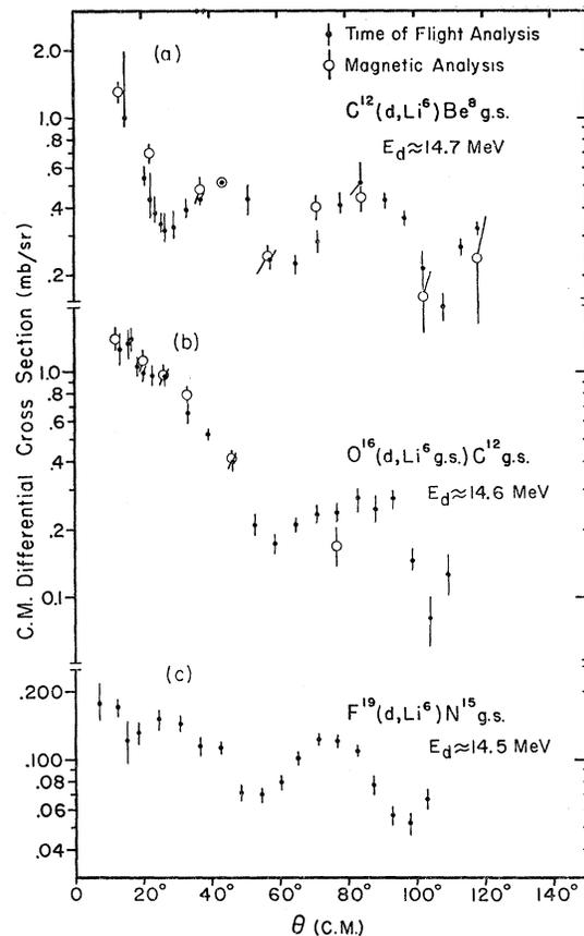
FIG. 8. Angular distributions, in the center-of-mass system, for three  $(d, Li^6)$  reactions. Time-of-flight data are indicated by solid dots, magnet data by open circles. Bars indicate relative experimental errors which are mostly, but not exclusively, due to statistics.
