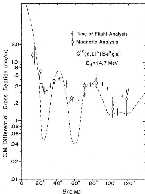
FIG. 9.  $\text{C}^{12}(d, \text{Li}^6)\text{Be}^8$  data compared with a DWBA calculation (Ref. 8), which assumed direct pickup of a preformed  $\alpha$  cluster (in zero range approximation). The theoretical curve is arbitrarily normalized.
