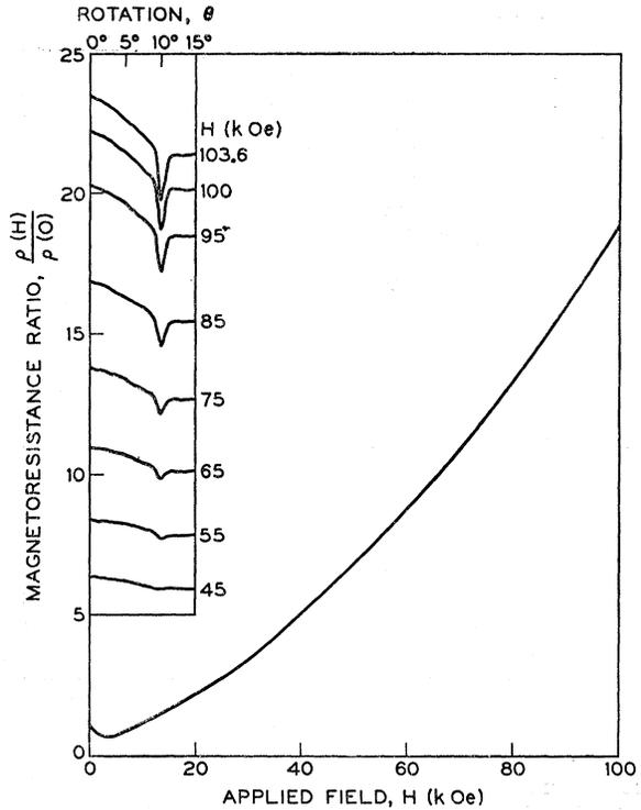
FIG. 3. Magnetoresistance of iron. The main diagram shows the field dependence of the magnetoresistance up to an applied field,  $H = 100$  kOe, when  $\mathbf{H}$  is directed along the minimum near  $[10\bar{1}]$  of the curve  $\varphi = 10^\circ$  of Fig. 1. The insert shows the latter curve in the neighborhood of the minimum for several values of  $H$ .
