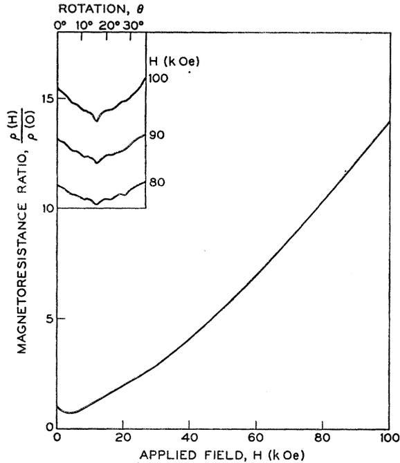
FIG. 4. Magnetoresistance of iron. The main diagram shows the field dependence of the magnetoresistance up to an applied field,  $H=100$  kOe, when  $\mathbf{H}$  is directed along the minimum at  $[001]$  for the  $\langle 110 \rangle$  sample. The insert shows the variation of the magnetoresistance with the rotation angle  $\theta$  in the neighborhood of the minimum for several values of  $H$ .
