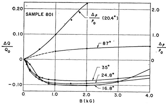
FIG. 3. Relative change of thermoelectric power  $\Delta Q/Q_0$  for sample 801 in transverse magnetic field in the classical region. The negative value of  $\Delta Q/Q_0$  observed near the liquid-hydrogen temperature range indicates that the phonon-drag contribution is small. The relative magnetoconductance at 20.4°K is also shown (vertical scale on the right).
