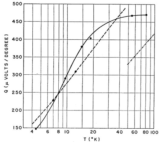
Fig. 2. Thermoelectric power of an  $n$ -type InSb sample (584) with carrier density  $4 \times 10^{14}$ /cc. The solid line represents a smooth curve through the experimental points marked by  $\bullet$ . The other two curves represent the theoretical values of the electronic contribution for different assumptions about the electron scattering: (i) dashed curve (---) for scattering on ionized impurities; (ii) dot-dash curve (- · -) for scattering on acoustic phonons.
