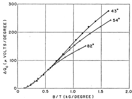
FIG. 4. Change of thermoelectric power in transverse magnetic field in the quantum region. On the  $y$  axis is plotted the increase in  $Q$  over the saturation value observed in the classical region (Fig. 3). The overlapping of curves for small values of  $B/T$  indicates negligible contribution from phonon drag. The divergence of the three curves for large  $B/T$  indicates that a measurable amount of phonon-drag contribution is realized.
