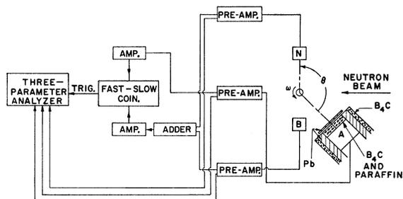
FIG. 2. Schematic diagram of the experimental arrangement. Crystal A was 16 in. from the center of the samples, crystal N was 12 in., and crystal B was 9 in. The lead in front of crystal A was about  $\frac{1}{4}$  in. thick.
