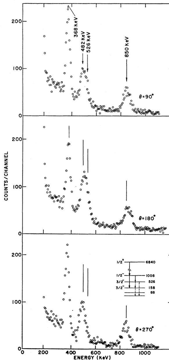
FIG. 5. Examples of the spectra in coincidence with gamma rays of about 5.83 MeV. These were used to determine the spin of the level at 1.008 MeV in  $\text{Ni}^{63}$ . For comments about the level scheme, see the caption for Fig. 4. An analysis of the line at 850 keV was used to determine the spin of the level at 1.008 MeV.
