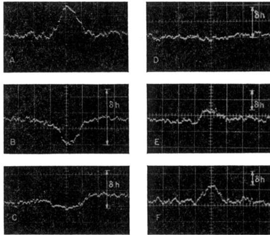
FIG. 1. Oscilloscope display of *F*-center absorption signal during recovery. *A* is the equilibrium signal and *B*, the signal immediately after inversion. *C*, *D*, *E*, and *F* photographed with increasing delay after inversion illustrate the gradual recovery of  $\delta h$  to zero. The sample was prepared by gamma irradiation and the measurements were taken at 4.2°K and 3.2 kOe. The *F*-center concentration was about  $4 \times 10^{16} \text{ cm}^{-3}$ .
