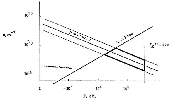
FIG. 3. Bounds of temperature and density for self-confined models, given by the requirement that the Coulomb-collision time ( $\tau_c$ ) and the radiation-losses time ( $\tau_R$ ) ought to be smaller than the observed lifetime (seconds), and that  $nkT \sim 1$  atm for mechanical equilibrium. These restrictions reduce the range of variation of  $T$  and ( $n$ ) to within the indicated trapezoid.
