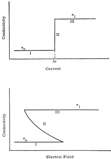
FIG. 4. Idealized plot of conductivity versus current density and electric field. The assumption of this behavior for  $\sigma$  allows us to find an exact nontrivial and physically interesting solution to the conduction-model equations.
