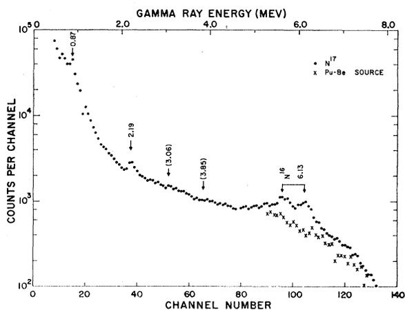
Fig. 2. NaI scintillation detector spectrum observed following the triton bombardment of a target of 99.5%  $N_2^{15}$ . Beta absorber: 3.9 g/cm<sup>2</sup> Al. Response of the NaI detector to neutrons from a Pu-Be source is also indicated.  $N^{16}$  is a contaminant activity.
