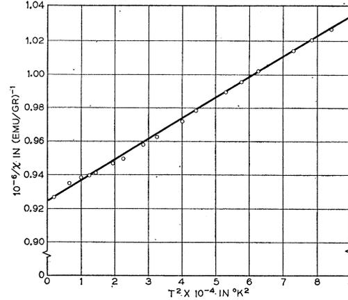
FIG. 4. The reciprocal of the mass susceptibility versus  $T^2$  using only the data above  $80^{\circ}\text{K}$  in the previous figure. The lowest temperature point is derived from the Knight shift found at  $20^{\circ}\text{K}$  as explained in the text.
