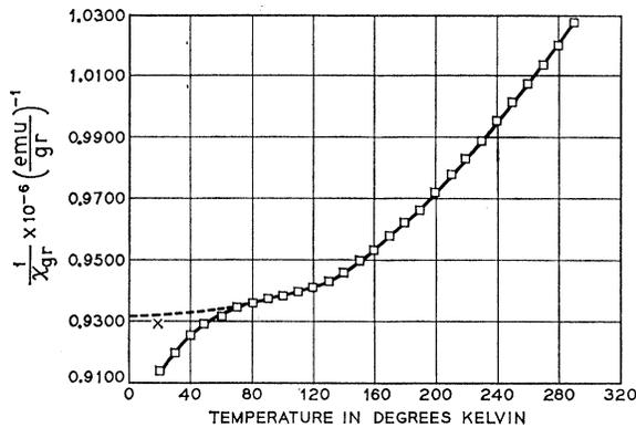
FIG. 3. The reciprocal of the mass susceptibility versus temperature is shown by the open squares. The point marked by a cross is the value of  $1/\chi$  determined using the Knight shift as a measure of the susceptibility in this low-temperature region. The dashed line is an extrapolation of the high-temperature  $1/\chi$  data subject to  $\partial(1/\chi)/\partial T = 0$ .
