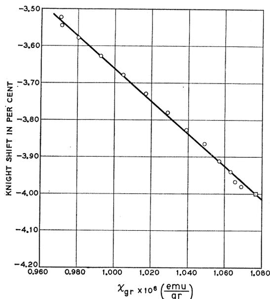
Fig. 1. The experimentally observed Knight shift of the  $\text{Pt}^{196}$  NMR in platinum metal versus the susceptibility, with temperature the implicit parameter, is shown by the open circles. The straight line is a best fit to this data. The open square is a low-temperature measurement of  $K$  which is arbitrarily placed on the straight line. The value of  $1/\chi$  corresponding to this is shown as a cross in Fig. 3.
