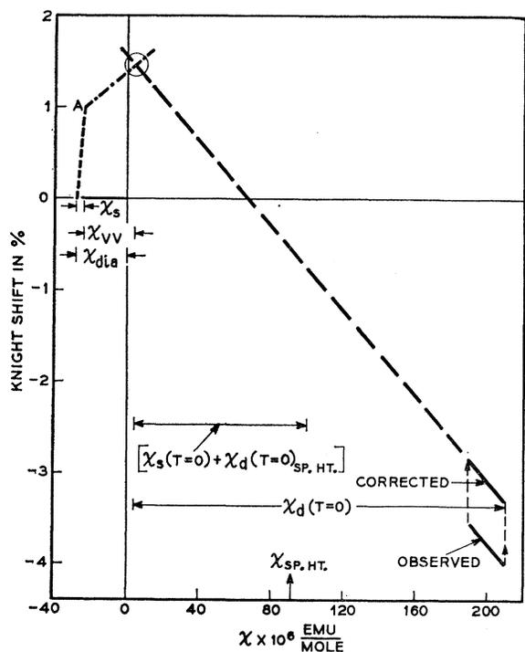
FIG. 2. A diagram of the Knight shift of the  $\text{Pt}^{195}$  NMR in platinum metal versus the susceptibility. The solid line marked "observed" is the experimental datum shown in Fig. 1, only much reduced because of the scale change. The solid line immediately above marked "corrected" is the same data corrected for the positive NMR shift in the chloroplatinic acid reference solution. The remaining features of the  $K$  versus  $\chi$  diagram are discussed in detail in the body of the paper.
