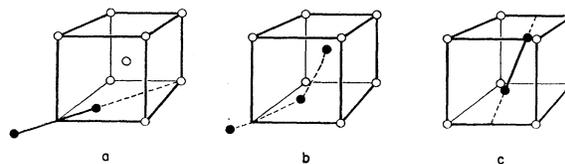
FIG. 4. The iron interstitial migration process. Configurations (a) and (c) are both  $I_2$  configurations, and (b) is  $I_7$ , the saddle point configuration.
