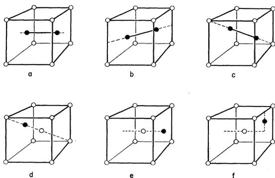
FIG. 3. Six iron interstitial configurations: (a)  $I_1$  or  $\langle 100 \rangle$  split interstitial; (b)  $I_2$  or  $\langle 110 \rangle$  split interstitials; (c)  $I_3$ ,  $\langle 111 \rangle$  split interstitial or crowdion; (d)  $I_4$  or activated crowdion; (e)  $I_5$  or octahedral interstitial; and (f)  $I_6$  or tetrahedral interstitial.
