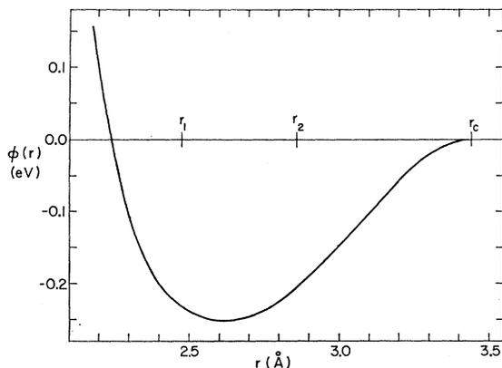
FIG. 2. The iron-iron interaction potential,  $\phi(r)$ , which was used in the present calculation.
