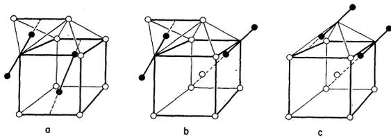
FIG. 5. The iron di-interstitial migration process. Configurations (a) and (c) are both stable di-interstitial configurations, and (b) is the intermediate step between (a) and (c).
