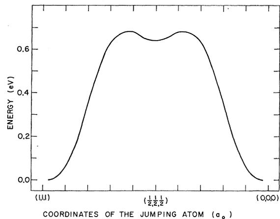
FIG. 6. The vacancy migration energy barrier. The energy of the configuration is shown as a function of the position of the jumping atom, as the vacancy migrates from  $(0,0,0)$  at the left to  $(1,1,1)$  at the right. The curve does not extend to  $(1,1,1)$  and  $(0,0,0)$  because the atom relaxes towards the vacancy.
