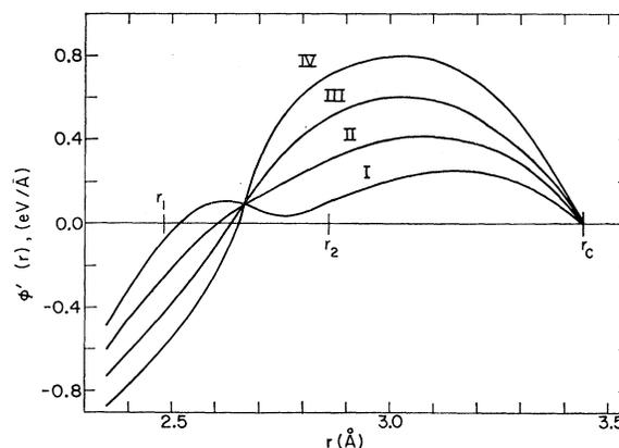
FIG. 1. A family of possible curves of the derivative of the potential,  $\varphi'(r)$ , which fit the short-range elastic constant conditions and which are zero midway between the second and third nearest neighbor distances.
