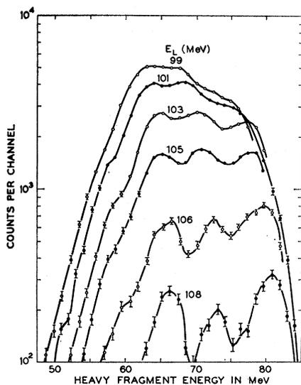
FIG. 1. Experimentally observed fine structure for the thermal-neutron-induced fission of  $U^{235}$  (from Ref. 1). Curves show the energy spectra of heavy fragments in coincidence with light fragments of the indicated energy.
