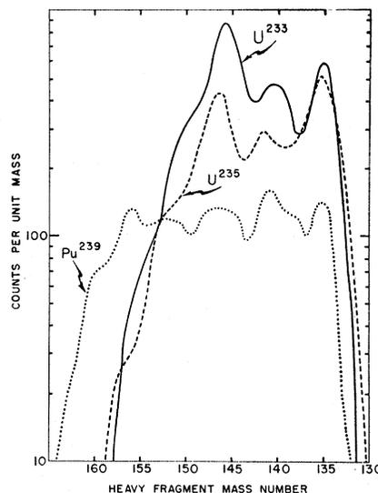
FIG. 2. Experimentally observed fine structure for the thermal-neutron induced fission of  $U^{233}$  (solid curve),  $U^{235}$  (dashed curve), and  $Pu^{239}$  (dotted curve). From Refs. 1 and 4. The data have been transformed to a coordinate system of counts per unit mass as a function of the mass of the heavy fragment. The light fragment kinetic energies are 108.7 MeV for  $U^{235}$ , 109.7 MeV for  $U^{233}$ , and 113.3 MeV for  $Pu^{239}$ .
