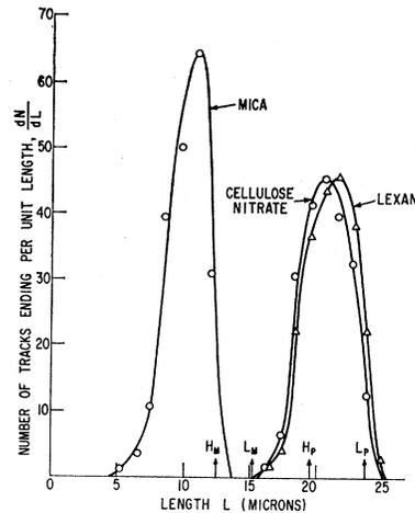
Fig. 5. Length distributions of fragments from the spontaneous fission of  $Cf^{252}$ , which have impinged at a  $20^\circ$  angle on three detectors. The arrows along the abscissa indicate the estimated ranges of light ( $Z=38$ ,  $A=95$ ) and heavy ( $Z=54$ ,  $A=139$ ) fragments in mica ( $L_M$ ,  $H_M$ ) and in the polymers ( $L_P$ ,  $H_P$ ).
