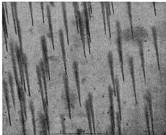
FIG. 4. Etched tracks of 139-MeV  $\text{S}^{32}$  ions entering Lexan polycarbonate at a  $30^\circ$  angle. The average track length is  $\sim 53 \mu$ , whereas the true range of the ions is estimated to be  $60 \mu$ . The micrograph was taken by transmitted light with the microscope focused below the surface of the tracks.
