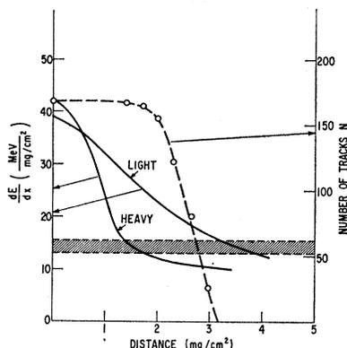
FIG. 3. Estimated curves of energy-loss rates of light ( $Z=38$ ,  $A=95$ ) and heavy ( $Z=54$ ,  $A=139$ ) fission fragments in Al. The shaded horizontal band represents the transition region for track detection in mica. The dashed line is obtained from the experimentally measured distribution of track lengths in mica (Fig. 5) and represents the number of tracks with a length greater than the value of the abscissa.
