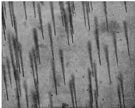
FIG. 4. Etched tracks of 139-MeV  $S^{32}$  ions entering Lexan polycarbonate at a  $30^\circ$  angle. The average track length is  $\sim 53 \mu$ , whereas the true range of the ions is estimated to be  $60 \mu$ . The micrograph was taken by transmitted light with the microscope focused below the surface on the ends of the tracks.
