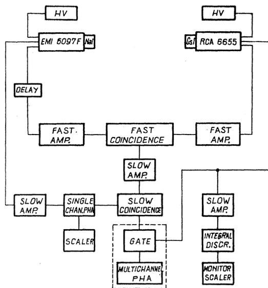
FIG. 1. Block diagram of the fast-slow coincidence circuit.
