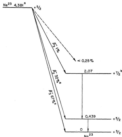
Fig. 2. Decay scheme for  $\text{Ne}^{23}$ . Energies are in units of MeV. Most of the data are taken from J. R. Penning and F. H. Schmidt, *Phys. Rev.* **105**, 647 (1957). See also (a) the present paper, (b) D. W. Braben, L. L. Green, and J. C. Willmott, *Proceedings of the Rutherford Jubilee International Conference* (Heywood and Company Ltd., London, 1961), p. 265.
