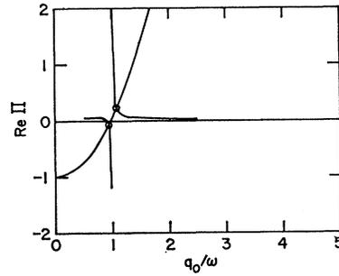
FIG. 13. Intersection of  $\text{Re}\Pi(q)$  and  $q_0^2 - \omega^2$  giving the phonon frequencies for fixed  $q$  in the limit  $q_0/|\mathbf{q}| \gg v_F$ .
