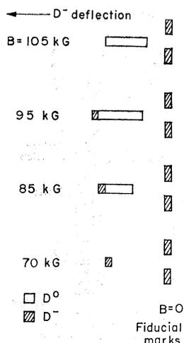
FIG. 4. Appearance of the data on an emulsion. The shaded regions have higher densities and are primarily  $D^-$  ions.
