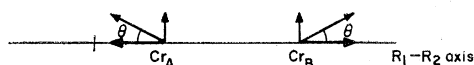
Fig. 8. Proposed molecular field configuration for a single pair. The net molecular field component perpendicular to the c axis is expected to spiral about the c axis as one moves along it so that there will be no net moment.
