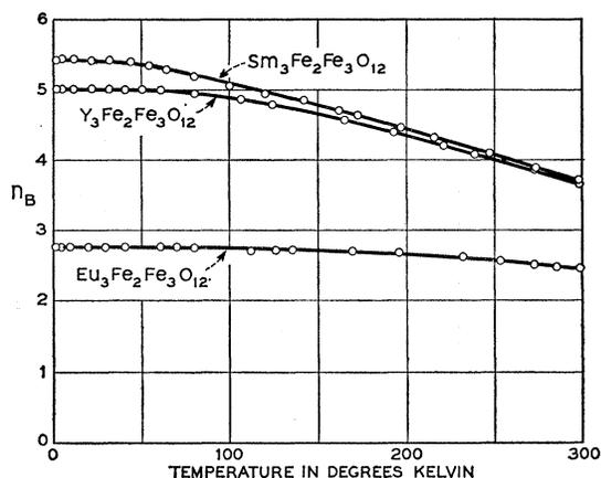
FIG. 4.  $n_B$  versus  $T$  for spherical crystals of samarium iron garnet and of europium iron garnet allowed to rotate freely in the applied field. Shown also is the curve for polycrystalline yttrium iron garnet. All specimens were saturated at field of 4.9 kOe or lower.
