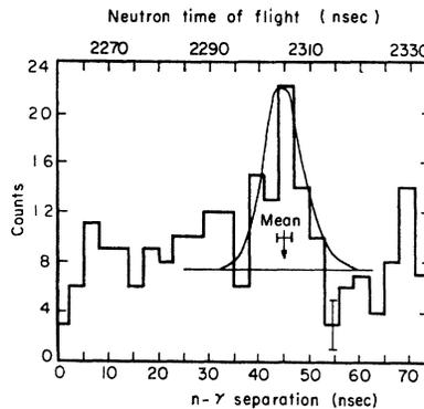
FIG. 9. Slow-neutron time distribution at 67 ft. Neutron  $PH \leq 0.8$  max;  $\gamma$   $PH \geq 0.32$  max. The reduction in minimum  $\gamma$   $PH$  compensates for the pulse-height attenuation in the delay cable.
