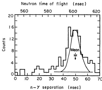
FIG. 7. Slow-neutron time distribution at 17 ft, Run II. Neutron  $PH \leq 0.8$  max;  $\gamma$   $PH \geq 0.40$  max. The beam level for this run was approximately one-half that of Run I.
