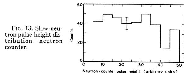
FIG. 13. Slow-neutron pulse-height distribution—neutron counter.
