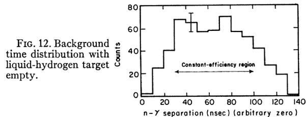
FIG. 12. Background time distribution with liquid-hydrogen target empty.
