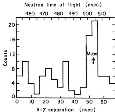
FIG. 11. Fast-neutron time distribution at 67 ft. Neutron  $PH \geq 0.92$  max;  $\gamma$   $PH \geq 0.46$  max.
