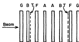
FIG. 2. Thin-target assembly. G, guard foil; B, backward catcher foil; T, target; F, forward catcher foil; A, activation foil.
