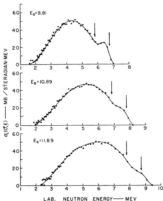
FIG. 3. Energy spectra of neutrons emitted at zero degrees from the D+T interaction for various deuteron bombarding energies,  $E_D$  (MeV). The arrow appearing at the higher neutron energy indicates the maximum possible energy of neutrons from the  $T(d, np)T$  reaction; the other arrow indicates the maximum possible energy of neutrons from the  $T(d, 2n)He^3$  reaction.
