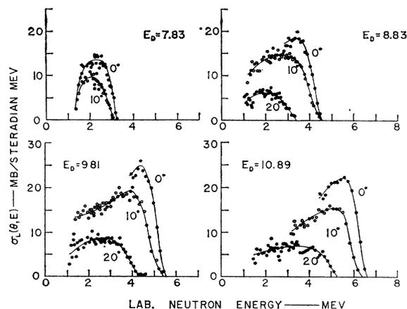
FIG. 10. Angular distributions of the neutron spectra for the D+H interaction for various deuteron bombarding energies,  $E_D$  (MeV).
