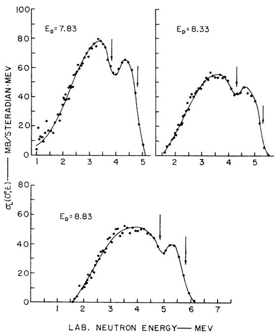
FIG. 2. Energy spectra of neutrons emitted at zero degrees from the D+T interaction for various deuteron bombarding energies,  $E_D$  (MeV). The arrow appearing at the higher neutron energy indicates the maximum possible energy of neutrons from the  $T(d, np)T$  reaction; the other arrow indicates the maximum possible energy of neutrons from the  $T(d, 2n)He^3$  reaction.
