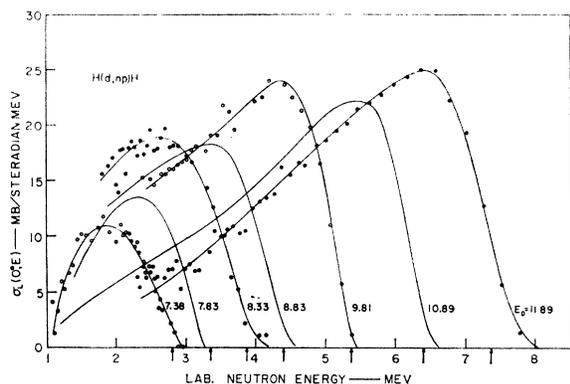
FIG. 9. Energy spectra of neutrons emitted at zero degrees from the D+H interaction for various deuteron bombarding energies,  $E_D$  (MeV). The arrows indicate for each spectrum the maximum possible energy of neutrons from the H( $d, n$ )pH reaction.
