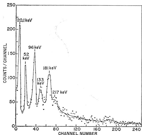
FIG. 4. The low-energy capture gamma-ray spectrum of rhodium in coincidence with the 52-keV line, with a  $\frac{3}{8}$ -in. tin plus  $\frac{1}{8}$ -in. copper filter between the rhodium sample and the "fixed" channel NaI(Tl) detector.
