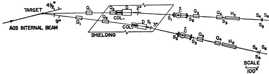
FIG. 1. Beam layouts for  $K^\pm p$  total cross-section measurements.  $K$  mesons were produced at the Brookhaven AGS in an internal target. The  $4\frac{1}{2}^\circ$  beam was used for measurements from 10 to 19 BeV/c, and the  $9^\circ$  beam for measurements from 3 to 12 BeV/c.
