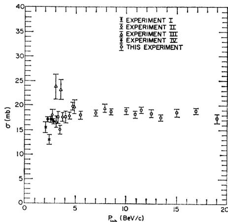
FIG. 8. Comparison of  $K^+ - p$  total cross sections with previous experiments. Experiment I: H. C. Burrowes *et al.* reference 5. Experiment II: A. S. Vovenko *et al.* (reference 6). Experiment III: G. von Dardel *et al.* (reference 9) Experiment IV: V. Cook *et al.* (reference 7).
