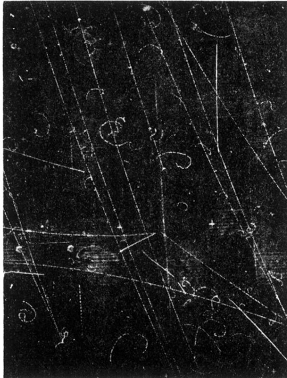
FIG. 2. The photograph shows a K^+ charge exchange followed by a \bar{K}^0 interaction. The \bar{K}^0 interaction produced by a \pi^+ and a \Lambda hyperon.
