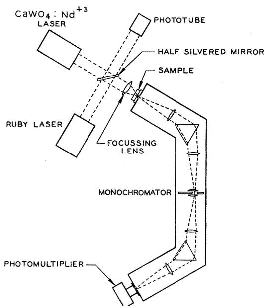
FIG. 1. Schematic drawing of experimental arrangement used for both the SHG of the  $\text{CaWO}_4:\text{Nd}^{3+}$  and ruby laser lines, and the mixing of these two laser beams. The focusing lens is a 20-mm focal length lens of variable aperture. The phototube is used to detect a portion of the laser fundamental which is then compared with the nonlinear signal output on a dual beam oscilloscope.
