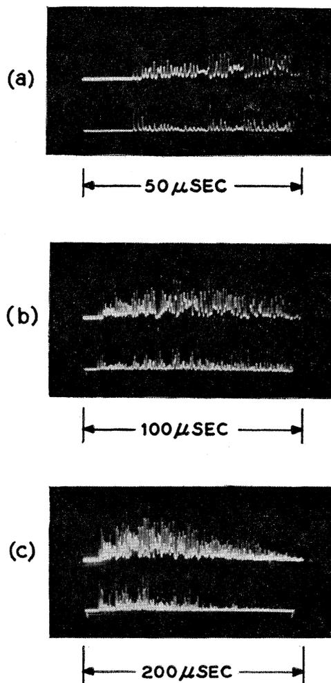
FIG. 2. Second harmonic generation of the  $\text{CaWO}_4:\text{Nd}^{3+}$  laser beam in KDP. In each frame, the upper trace shows the fundamental, and the lower trace the second harmonic.
