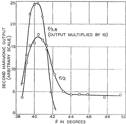
FIG. 3. Second harmonic output of the  $\text{CaWO}_4:\text{Nd}^{3+}$  laser beam in KDP as a function of the angle  $\theta$  between the optic axis in the crystal and the focused laser light cone. The value of  $\theta$  at the intensity maximum is seen to be the same for the  $f/2$  focusing lens as for the same lens stopped down to  $f/5.6$ .
