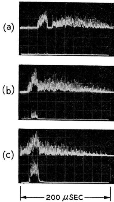
FIG. 4. Mixing of the pulsed ruby and  $\text{CaWO}_4:\text{Nd}^{3+}$  laser beams in KDP. In each frame the upper trace shows the laser outputs and the lower the mixed sum frequency output at 4189 Å. In (a), the two lasers are out of phase timewise (the ruby laser pulse, approximately 20  $\mu\text{sec}$  long, occurs first) and no mixed signal is generated. When the two lasers overlap timewise as in (b) and (c), a mixed signal output is observed.
