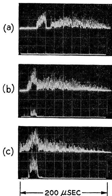
FIG. 4. Mixing of the pulsed ruby and  $\text{CaWO}_4:\text{Nd}^{3+}$  laser beams in KDP. In each frame the upper trace shows the laser outputs and the lower the mixed sum frequency output at  $4189 \text{ \AA}$ . In (a), the two lasers are out of phase timewise (the ruby laser pulse, approximately  $20 \mu\text{sec}$  long, occurs first) and no mixed signal is generated. When the two lasers overlap timewise as in (b) and (c), a mixed signal output is observed.
