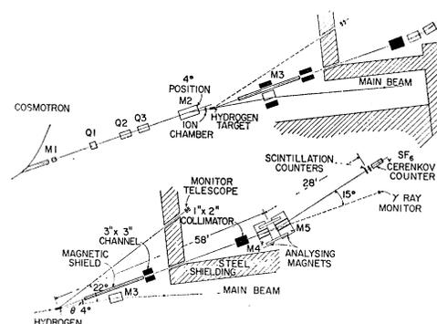
FIG. 3. Experimental arrangement. The upper drawing indicates the over-all trajectory of the beam, starting from the Cosmotron; the lower drawing shows the setup downstream from the target.  $M$  refers to bending magnets;  $Q$  to quadrupole magnets.
