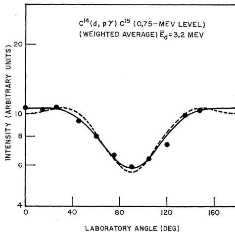
FIG. 4. Angular distribution of the  $C^{15}$  0.75-MeV  $\gamma$ -ray for an average deuteron energy of 3.2 MeV. The solid curve is a least squares fit to the experimental points,  $W(\theta, E_d)$ . The dashed curve is the prediction of plane-wave stripping theory (reference 1) for a  $\frac{5}{2}^+ \rightarrow \frac{1}{2}^+$   $\gamma$ -ray transition (see text).
