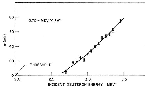
FIG. 6. The total cross section for the  $C^{14}(d,p)C^{15}$  (0.75-MeV level) reaction as a function of deuteron energy. The total cross section scale (ordinate), which has an uncertainty of 30%, was obtained from the yield and angular distribution of the 0.75-MeV  $\gamma$  rays (see text).
