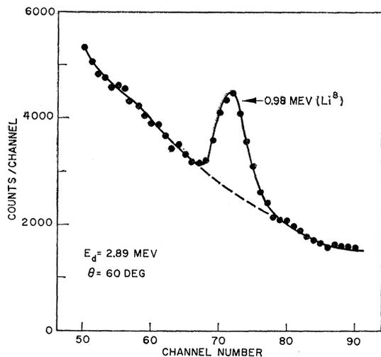
FIG. 2. A pulse-height spectrum showing the total absorption peak of the 0.98-MeV  $\gamma$  ray from the  $\text{Li}^7(d,p\gamma)\text{Li}^8$  reaction at a deuteron energy of 2.89 MeV. The spectrum was obtained with a 2-in. diam by 2-in. long NaI(Tl) crystal at  $60^\circ$  to the deuteron beam.
