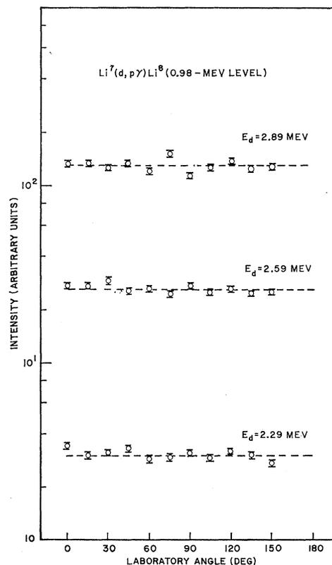
FIG. 7. Angular distributions for the  $Li^8$  0.98-MeV  $\gamma$  ray. The dashed curves represent an isotropic distribution, which would be indistinguishable on the plot from the distribution predicted from plane-wave stripping theory for a  $1^+ \rightarrow 2^+$   $\gamma$ -ray transition with a channel spin ratio  $(s=2)/(s=1)$  equal to 3.3 (see text).
