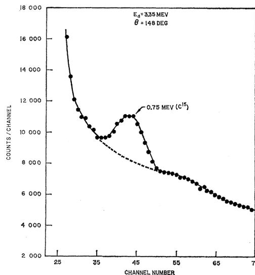
FIG. 1. A pulse-height spectrum showing the total absorption peak of the 0.750-MeV  $\gamma$  ray from the  $\text{C}^{14}(d,p\gamma)\text{C}^{15}$  reaction at a deuteron energy of 3.35 MeV. The spectrum was obtained with a 1-in. diam by 1-in. long NaI(Tl) crystal at 148° to the deuteron beam.
