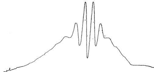
FIG. 2. A typical "Ramsey" pattern of the  $\Delta F = \pm 1$  field-independent transition with  $180^\circ$  phase difference between loops. The frequency difference between the two maxima is about 2.6 kc/sec.
