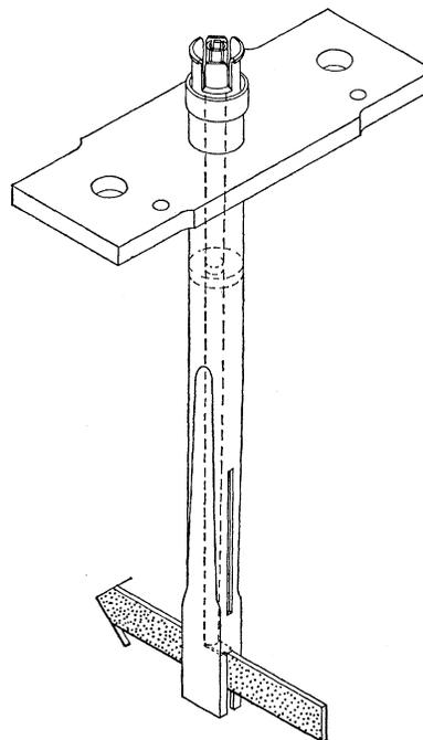
FIG. 1. Loop producing the oscillatory field parallel to the steady  $C$  field for inducing  $\Delta F=0$  transitions. The principal conductor producing the fields is the termination between the lower end of the central conductor and the right-hand side of the outer conductor.
