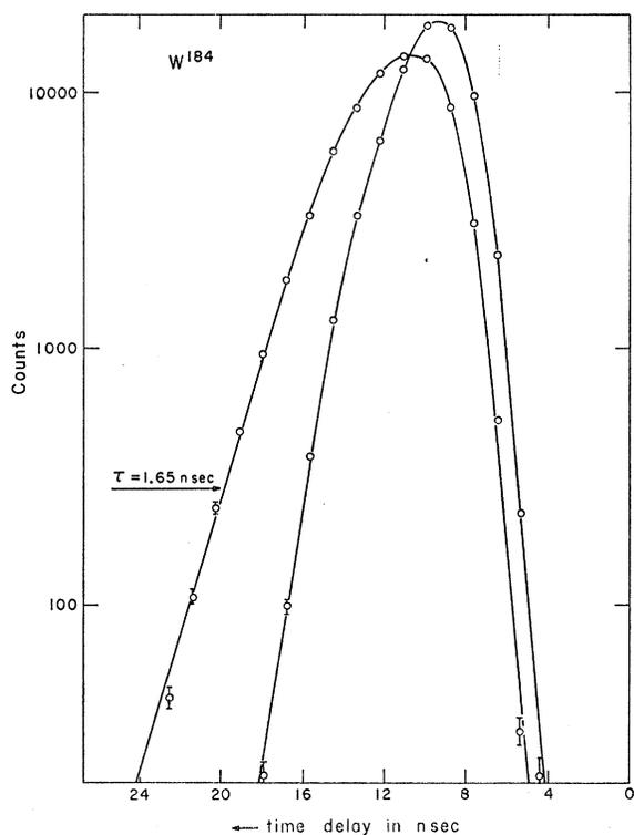
FIG. 2. Time distribution of pulses for the 111-kev radiation from a W<sup>184</sup> target compared with "prompt" radiation from the 110-kev transition in Tm<sup>169</sup> normalized to the same number of total counts.
