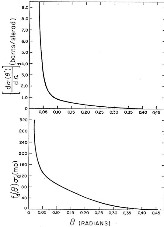
FIG. 6. The upper curve is  $[d\sigma(\theta')/d\Omega]$  for carbon with  $V_R=32.5$  Mev and  $V_I=40$  Mev, as calculated by Loki. The lower curve is  $f_d(\theta)\sigma_d$ , calculated from Eq. (4) for carbon with  $V_R=32.5$  Mev and  $V_I=40$  Mev.
