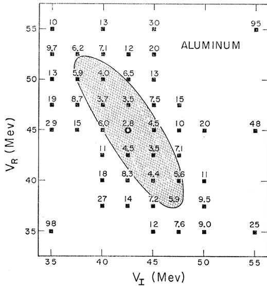
FIG. 8. Contour graph of  $S$  [see Eq. (5)] as a function of  $V_R$  and  $V_I$  for aluminum. The solid curve represents the  $S=6$  contour. The correct  $V_R$  and  $V_I$  pair should lie within the shaded portion.
