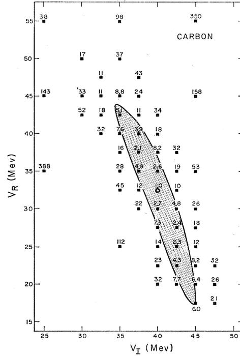
FIG. 7. Contour graph of  $S$  [see Eq. (5)] as a function of  $V_R$  and  $V_I$  for carbon. The solid curve represents the  $S=6$  contour. The correct  $V_R$  and  $V_I$  pair should lie within the shaded portion.
