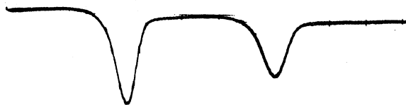
FIG. 2. N^{14} Zeeman resonances in the F=5/2 and F=3/2 states as observed in a field of 0.1 gauss.
