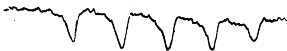
FIG. 3. Quadratic splitting of the N^{14} F=5/2 Zeeman resonance into its five components in a field of 1.0 gauss.
