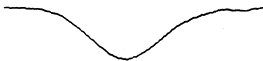
FIG. 4. Single Zeeman component of the N^{14} hyperfine transition between the F=5/2 and F=3/2 states. The sweep time is 0.2 sec.
