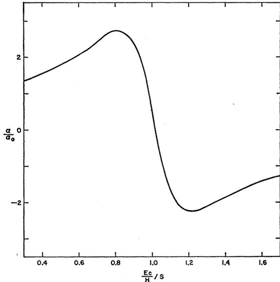
FIG. 1. Plot of bracketed term in Eq. (12) for the following values of parameters:  $D=1$  cm<sup>2</sup>/sec,  $\tau_r=10^{-8}$  sec,  $k=10^4$  cm<sup>-1</sup>,  $s=10^6$  cm/sec.
