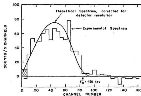
FIG. 4. Net positron spectrum of  $K^{40}$ .
