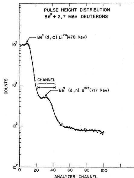
FIG. 4. Pulse-height distribution in the plastic scintillator from the deuteron bombardment of Be. The single channel discriminator was channeled as shown on the 717-keV gamma from Be<sup>9</sup>(*d,n*)B<sup>10\*</sup>.
