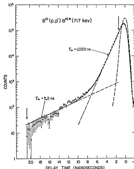
FIG. 7. Time spectrum of 717-keV gammas from the proton bombardment of boron. The faster component is attributed to the  $\text{B}^{10}(p,p')\text{B}^{10*}$  (717-keV) reaction. The full curve is a least-squares fit to the sum of two exponential decays in the region indicated by the arrows. Also shown is a prompt comparison curve obtained using gammas from the  $\text{Al}^{27}(p,p')\text{Al}^{27*}$  reaction.
