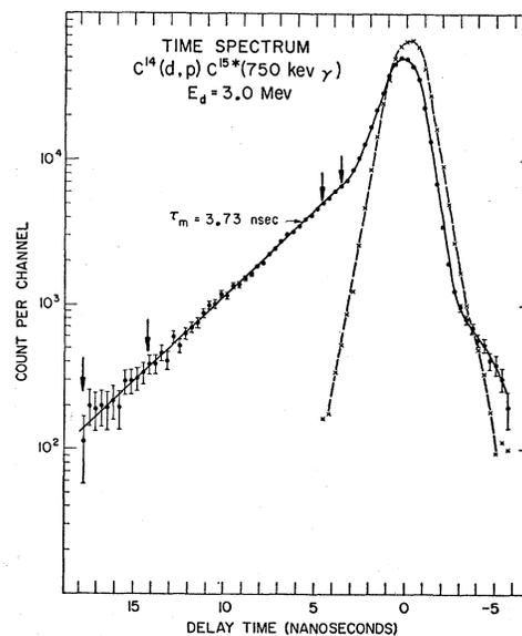
FIG. 9. Time spectrum of 750-kev gammas from  $C^{14}(d,p)C^{15*}$ . The exponential part of the decay is a least squares fit to the region of the data indicated by the arrows. Also shown is a prompt comparison curve using gammas from the  $C^{12}(d,p)C^{13*}$  reaction.
