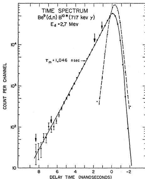
FIG. 6. Time spectrum of 717-keV gammas from  $\text{Be}^9(d,n)\text{B}^{10*}$ . The exponential part of the decay is a least squares fit to the region indicated by the arrows. Also shown is a prompt comparison curve obtained using gammas from the  $\text{C}^{12}(d,p)\text{C}^{13*}$  reaction.
