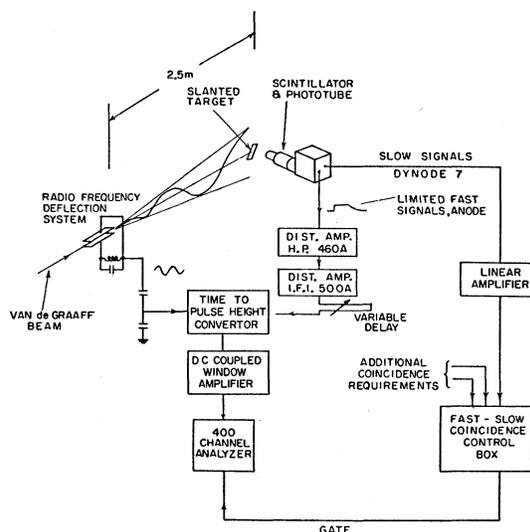
FIG. 3. Schematic diagram of the electronic equipment.
