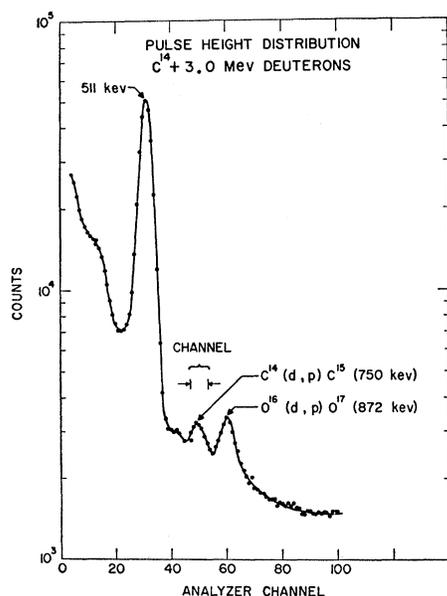
Fig. 5. Pulse height distribution in the NaI scintillator from the bombardment of  $C^{14}$  with 3-Mev deuterons. The single channel discriminator was channeled on the 750-kev gamma photopeak as shown.
