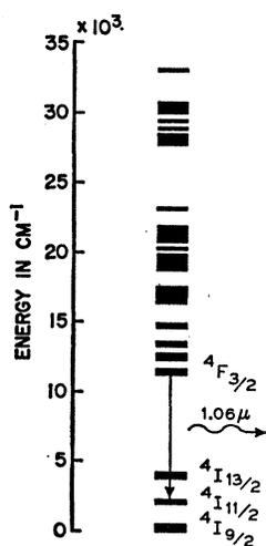
FIG. 1. Energy level diagram of  $\text{Nd}^{3+}$  in  $\text{CaWO}_4$ .
