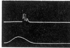
FIG. 3. Stimulated emission near threshold in  $\text{CaWO}_4:\text{Nd}^{3+}$  at  $1.065 \mu$ , approximately  $85^\circ\text{K}$ . Pumping is achieved by a linear FT 91 xenon flash lamp in a nonfocused single ellipse configuration. Lower trace: Variation of lamp intensity with time. Upper trace: Fluorescence and stimulated emission. Time increases to the right ( $50 \mu\text{sec}$  per division) and the traces are triggered simultaneously.
