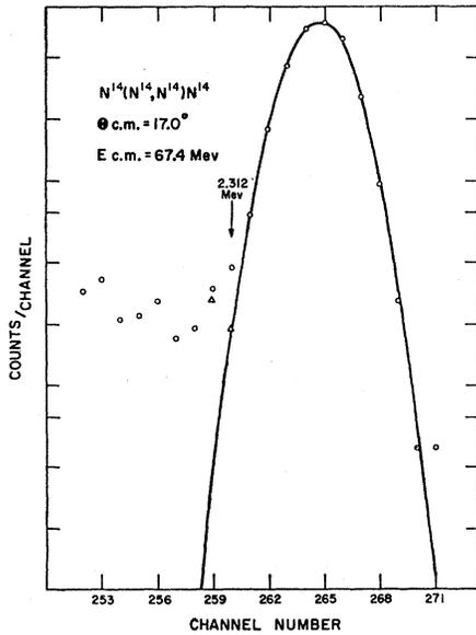
FIG. 4. A portion of the detector energy spectrum for the  $N^{14}-N^{14}$  reaction. The peak, due to elastic scattering, is shown with a resolution sufficient to eliminate the first excited state of  $N^{14}$  indicated by the arrow. The triangles represent the hypothetical value of the background count in their respective channels.
