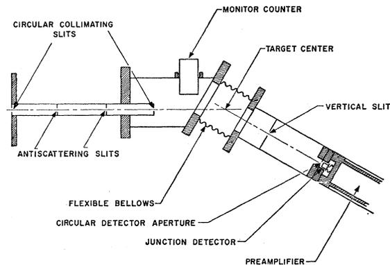
Fig. 1. A schematic view of the experimental apparatus in the plane of scattering. This differs from that shown in reference 9 only in the detector assembly.
