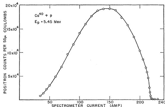
FIG. 4. Uncorrected spectrum of continuous distribution of positrons from pairs from the 3.35-Mev excited state of  $Ca^{40}$ .
