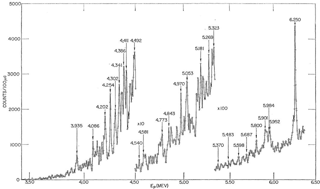
FIG. 10. Excitation function for population of the first excited state of  $Zr^{90}$  by proton bombardment.
