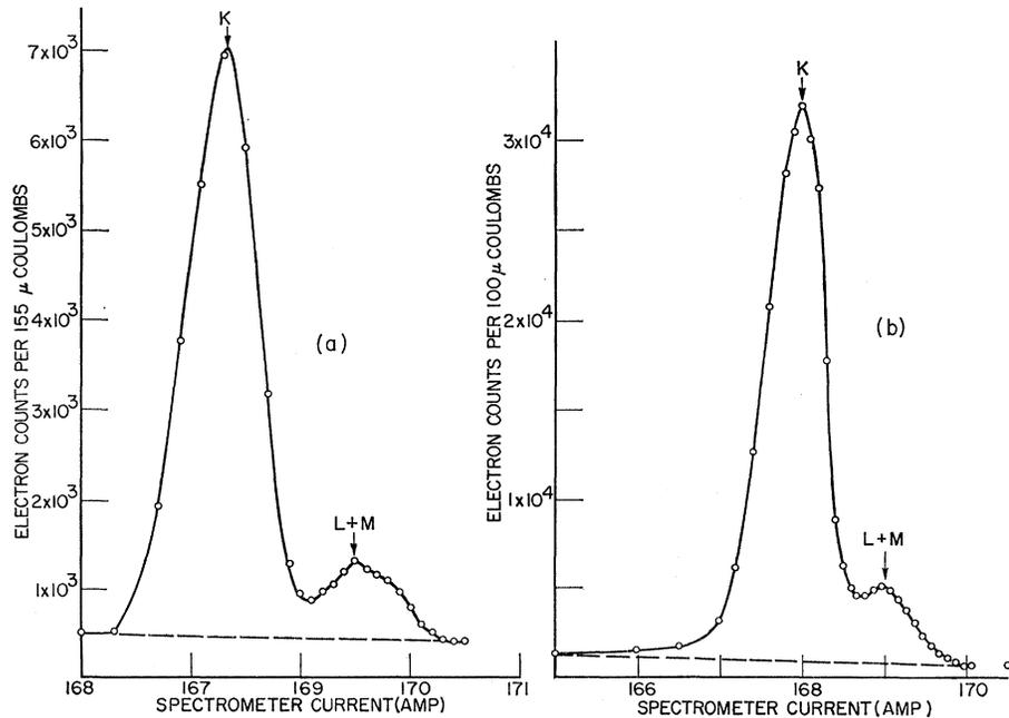
FIG. 15. (a) Spectrum of  $K$  and  $L+M+N+O$  conversion electrons from the 1.76-Mev excited state of  $Zr^{90}$  (1-mg/cm<sup>2</sup> target). (b) Spectrum of  $K$  and  $L+M+N+O$  conversion electrons from the 1.76-Mev excited state of  $Zr^{90}$  (2-mg/cm<sup>2</sup> target).
