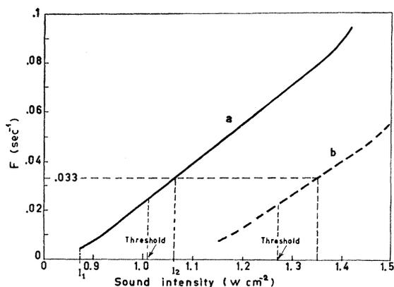
FIG. 3. Inverse of average delay of cavitation onset in distilled water; a sound field of constant intensity is applied to the liquid. (a) Unscreened tank; (b) 20-mm lead screen surrounding the tank.
