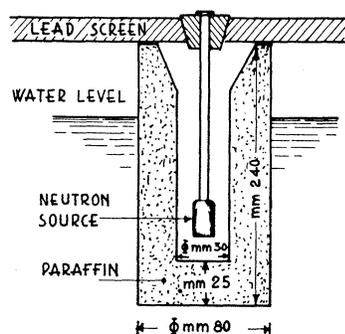
FIG. 11. Paraffin enclosure used for slowing down neutrons.
