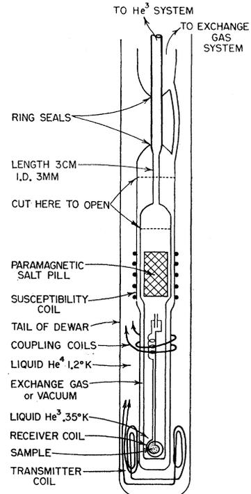
FIG. 1. Schematic drawing of the He<sup>3</sup> cryostat. The thermal link between the salt pill and the sample is discussed in the text.
