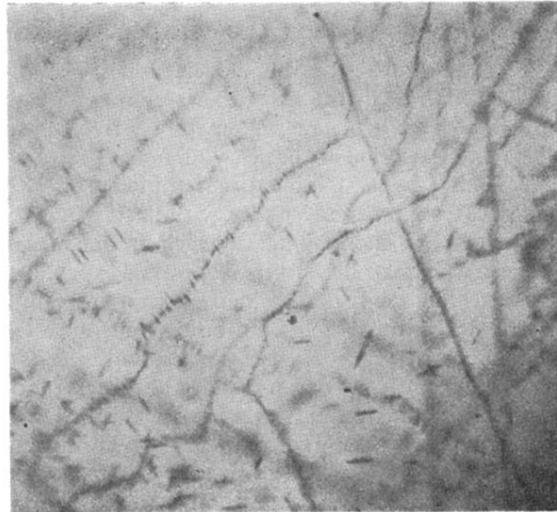
FIG. 6. Photograph of precipitate in ZnS:Ag crystal achieved by diffusion of copper. View parallel to hexagonal axis, field 75 \times 70 \mu . Depth of focus less than 1 \mu .
