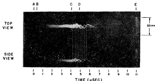
FIG. 1. Stereoscopic streak photographs of the plasma compression and  $m=2$  instability mode with  $-3$  kilogauss initial reverse field. (A) Start of discharge; (B) imploding shock reflects off axis; (C) onset of instability; (D) fission into two well-defined filaments; (E) imploding shock wave at beginning of the second half-cycle. The camera slit is imaged to the left of the photograph and defines the relative positions of the two filaments in the side and top views.
