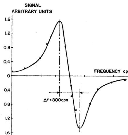
FIG. 16. Line shape of optically detected 0-0 transition in Cs<sup>133</sup>.
