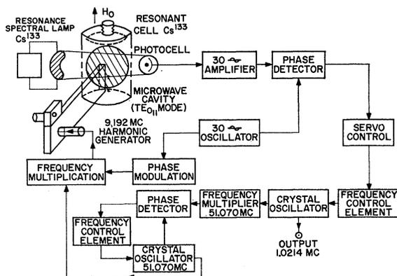
FIG. 1. Experimental arrangement.
