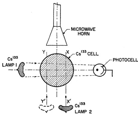
FIG. 17. Double light beam experimental arrangement for investigation of light intensity frequency shifts in a large resonance cell ( $XX'$  and  $YY'$  represent planes along which auxiliary resonance radiation from lamp 2 is focused).
