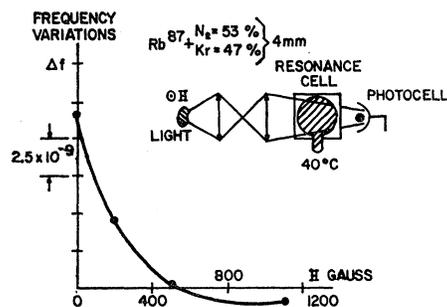
FIG. 19. Light-intensity frequency shifts as a function of magnetic field intensity at the light source: The magnetic field in displacing slightly the hyperfine components of the light source, as compared to the hyperfine components in the resonance cell, can change the magnitude or the sign of the light-intensity frequency shift.
